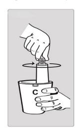
Step 3: Adjust bolus volume for Plugs E or F: insert Key D into sleeve of Upper Cap C and turn the Plug. To achieve desired volume, align scale line on the Key D with the edge of the sleeve.
